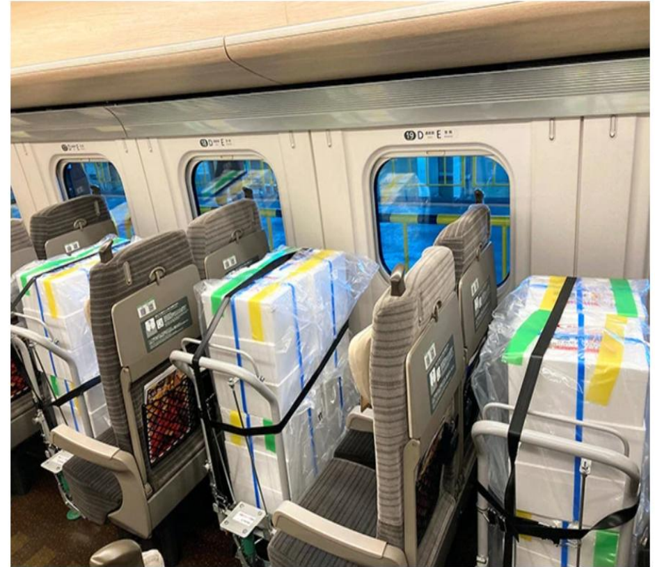
Parcels of goods are loaded onto trucks that fit between the seats aboard a Shinkansen. (Provided by East Japan Railway Co.)
