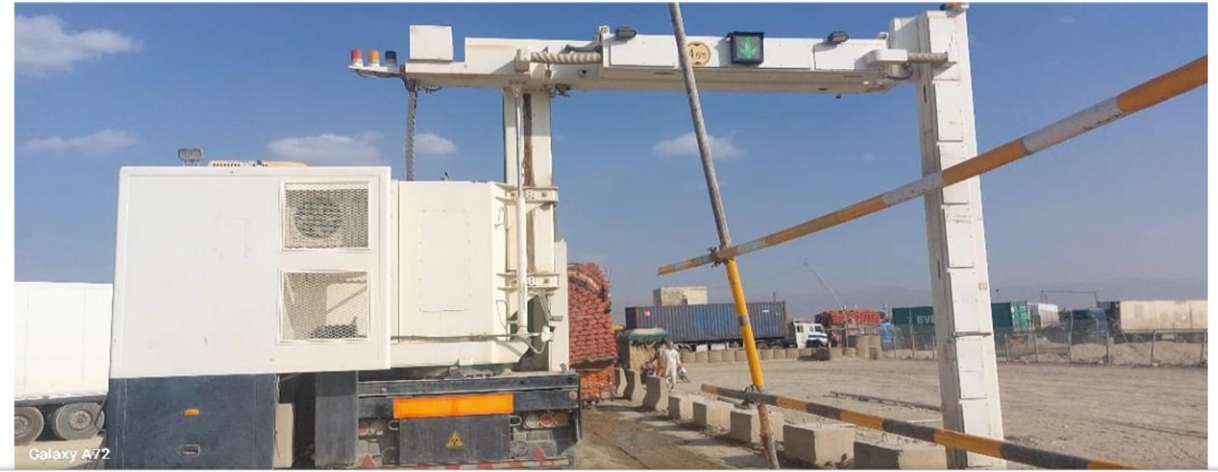
Drive Through Scanner NLC Terminal Yard
