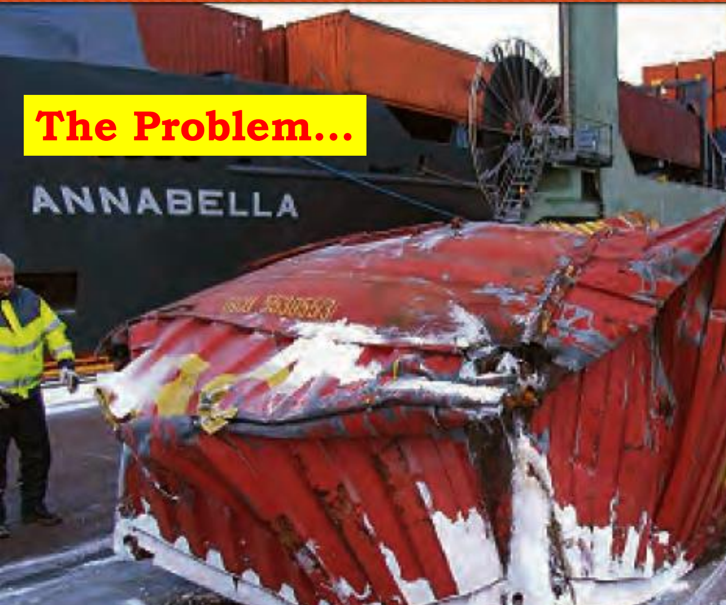
Baltic Sea 2007 - A stack of 7 containers toppled during rough weather. The upper containers (not shown) were tank containers fully loaded with butylene gas (IMDG Class 2.1)
